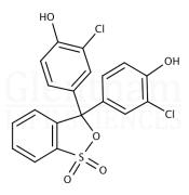
Property Specification Physical Description Red to green, red-brown or brown powder or crystals Solubility (0.1% in ethanol) Clear, orange, dark orange or red-orange solution pH Transition Range(s) 4.6 - 7.3 (yellow to purple) Wavelength of Maximum Absorption (λmax) 573.0 - 577.0 nm (0.1M NaOH) Absorptivity (1%/1cm) ≥ 1500 (\lambdamax, dried basis) ≤ 8.0% (1hr at 110 °C) Loss on Drying Assay (spectrophotometry) ≥ 90.0%
