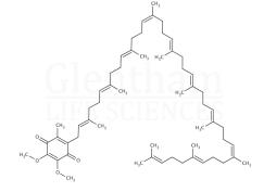
Property Specification Physical Description Yellow to dark orange powder Identification A, B according to USP Solubility (5% in chloroform) Clear to very slightly hazy, yellow to orange solution Water ≤ 0.1% Residue on Ignition Heavy Metals ≤ 20ppm Related Substances (TLC) Any Single Impurity: ≤ 0.5% Total Impurities: ≤ 1.0% 98.0 - 101.0 % (dried basis) USP Pharmacopoeia Specification(s)
