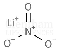
PropertySpecificationPhysical DescriptionWhite powder or crystalsSolubility (5% in water)Clear, colourless solutionLoss on Drying≤ 2.0%Assay (Titration)98.0 - 102.0 %
