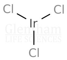
PropertySpecificationPhysical DescriptionDark green to brown or grey powderIridium (Ir) $\geq 63.0\%$ Trace Metals $\leq 2500$ ppmPurity (Trace Metals Basis) $\geq 99.8\%$
